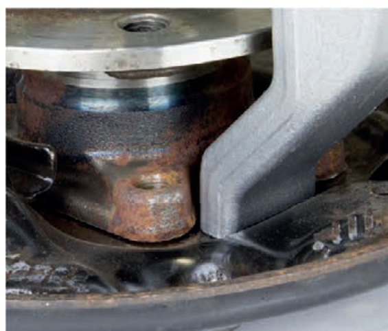
The press feet's get access to the small surfaces close to the bearing, pressing on the knuckle behind the brake shield.
