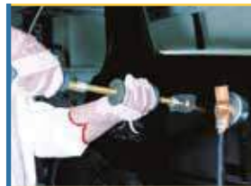
Spot hammer welding
